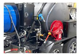
Water system controls moutned near control box and jetter reel for user-friendly layout.
