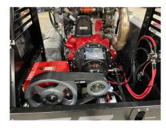
An enclosed engine compartment gives this jetter a clean look with user-friendly access for engine and water pump maintenance.
